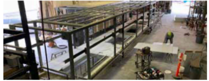
The elevator is manufactured horizontally making quality control a snap. This makes the structure and rails plumb and straight all the time.
